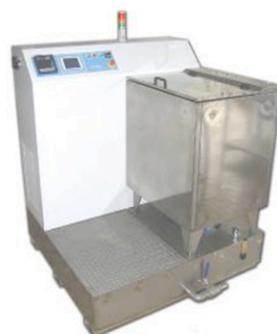
Suitable for performing the test envisaged by the **UNI EN ISO 10545-12** (ceramic tiles) and **UNI EN 1348** (adhesives for tiles) standards.
