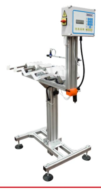
AUTOMATIC BELTS COVER is a device suitable to protect the glazing line belts that are placed under the Veil and Bell application, through the deviation to the recovery tank of the glaze coming from the application machine.
